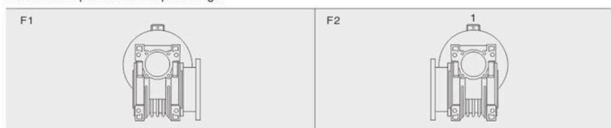
Position of motor joint box (viewed from the fan of the motor)
